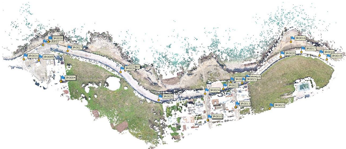
Fig. 3. Distribution of the GCPs implemented in the sparse points cloud
